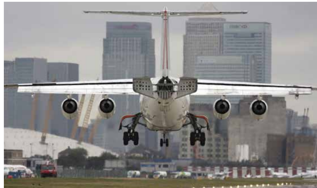
Air brakes in use on the BAe 146.
